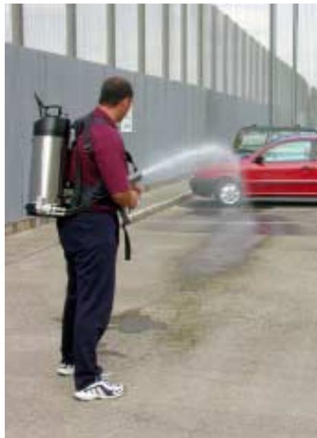
**FIGURE 5: Portable Water Cannon**
